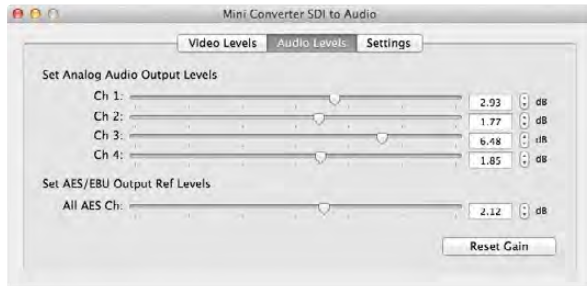
Adjust audio levels using Blackmagic Converter Utility.
