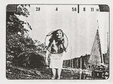
7 Check whether the exposure meter needle is within the proper range.
