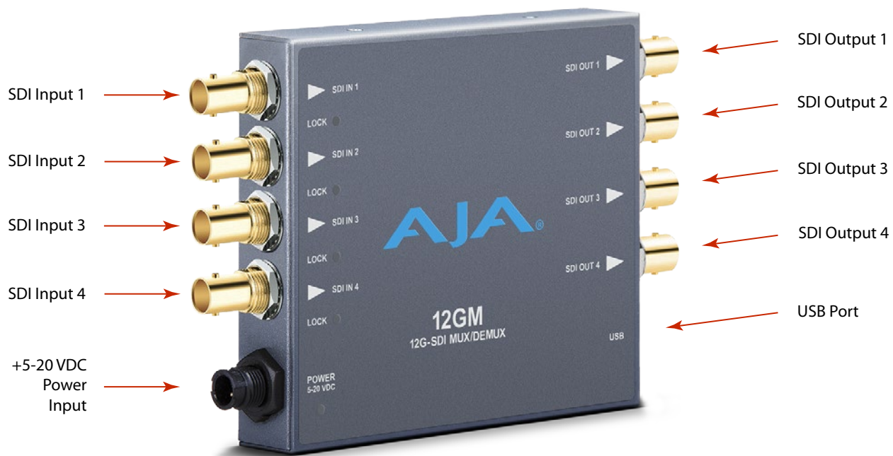
Figure 2. 12GM Converter Connections
